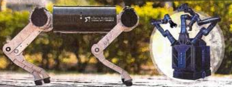
A quadruped robot by xTerra Robotics, which provides solutions for inspection, security and industrial tasks. (Inset) CynLr is a mobile system with three seven-axis arms created by CynLr, which focuses on teaching robots to recognise and handle unfamiliar objects
