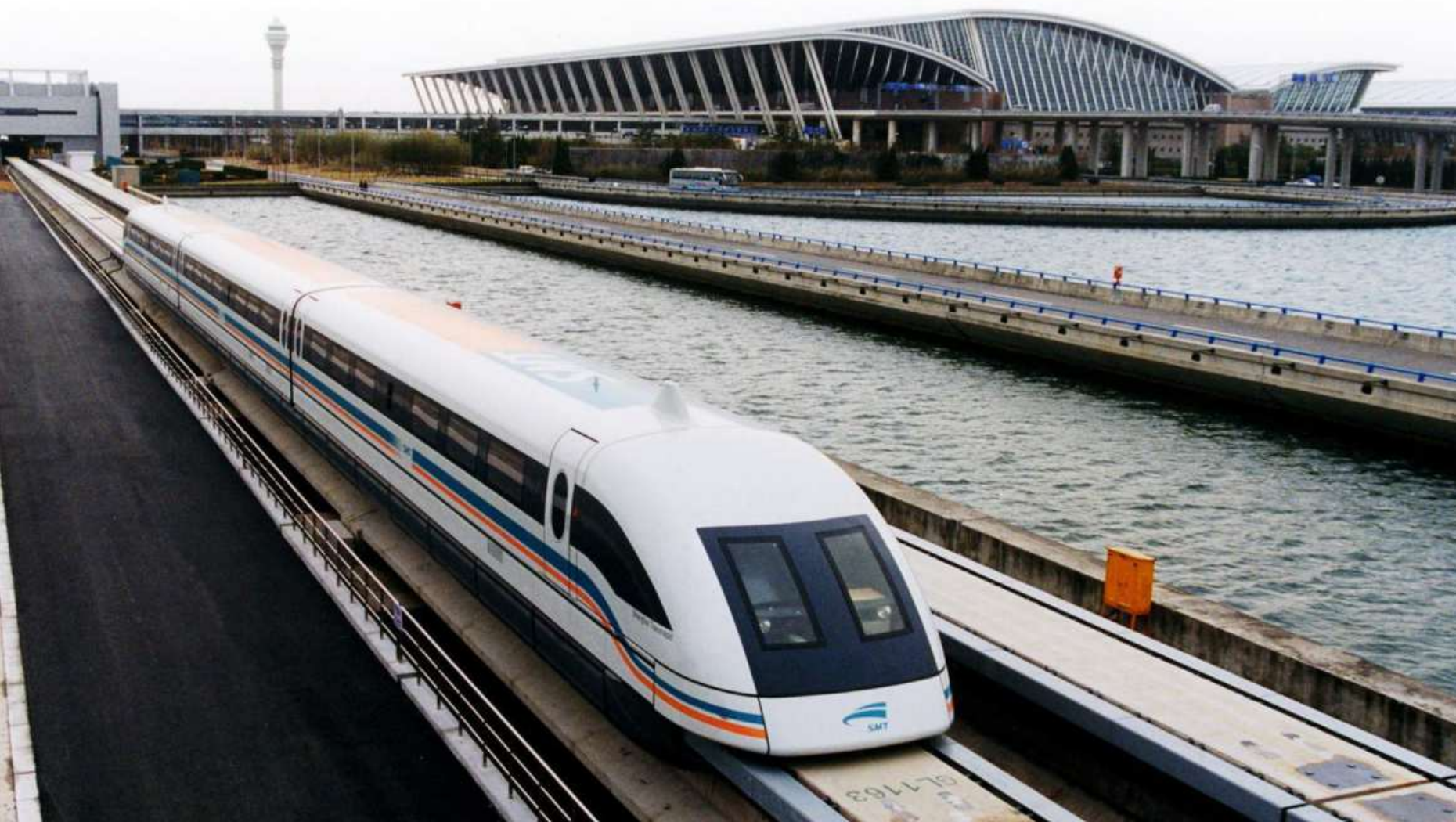
Engineers get the train to float above the tracks using electromagnetic suspension. SPECIAL ARRANGEMENT
