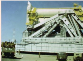
The Soviet Energia super-heavy booster being rolled to its launch pad in 1987. Designed to haul about 100 t to orbit, the program ended after only two flights, highlighting how economic factors can end even the biggest rockets.
