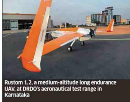
Rustum 1.2, a medium-altitude long endurance UAV, at DRDO's aeronautical test range in Karnataka
