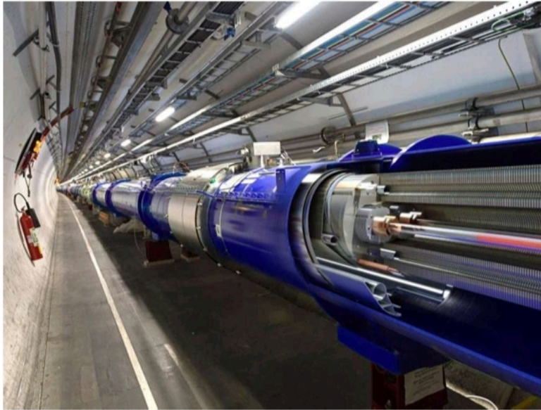
The Large Hadron Collider is the world's largest, most powerful particle accelerator. It accelerates particles, mainly protons, to near the speed of light in opposite directions around a 27-km underground ring. Then the particles are made to collide at four locations, where massive detectors collect data on what happens during the collision. CERN
